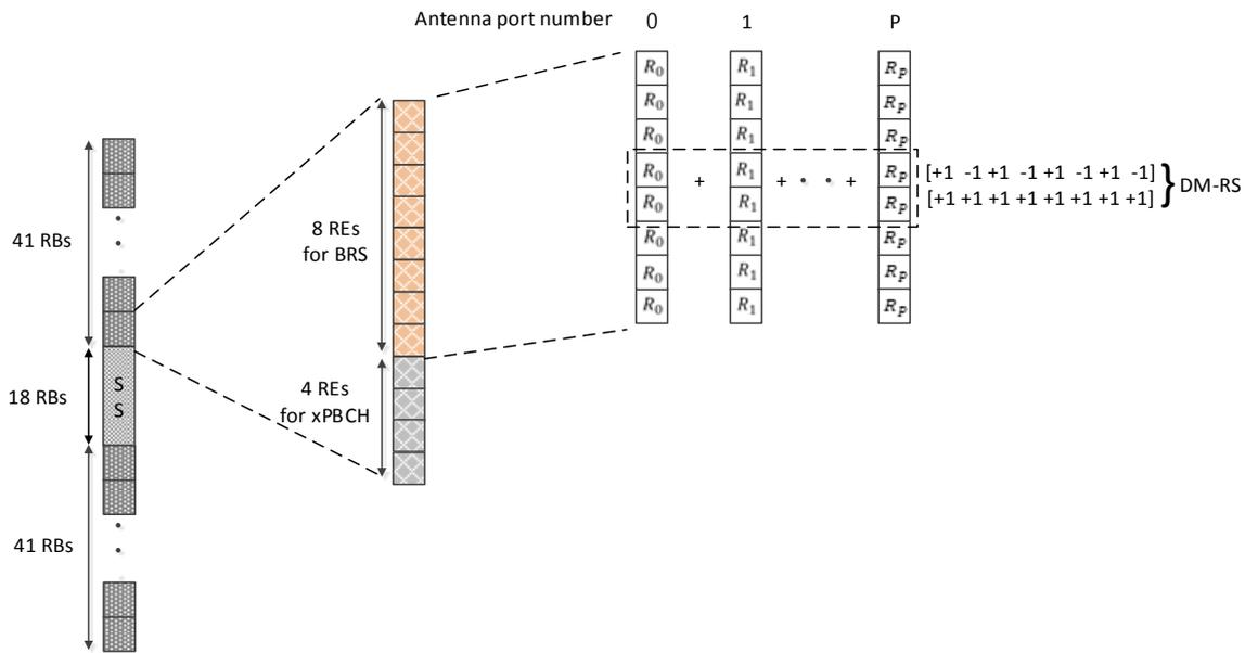
Figure 6.7.4.2-1. Mapping of beam reference signals including xPBCH and DM-RS
