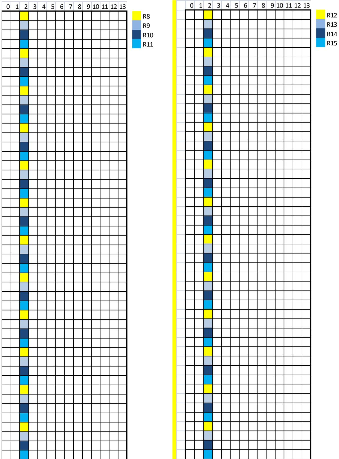
Figure 6.7.2.2-1: Mapping of UE-specific reference signals, antenna ports 8, 9, 10, 11, 12, 13, 14 and 15.
