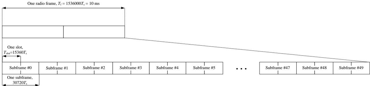
**Figure 4.2-1: Frame structure**
