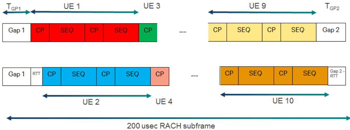
Figure 5.7.1-2: Reception of RACH signal at BS during RACH subframe
