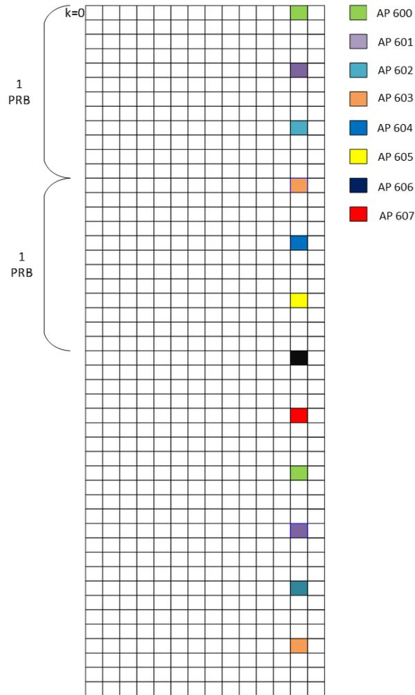
Figure 6.7.5.2-1: Mapping of BRRS showing a 1 symbol allocation, e.g.  $l=12$
