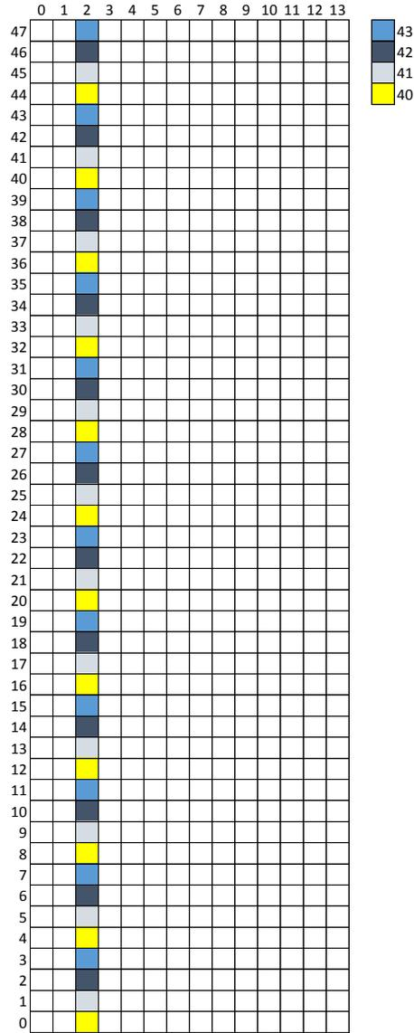
Figure 5.5.3.2-1: Mapping of UE-specific reference signals, antenna ports {40, 41,42,43}.
