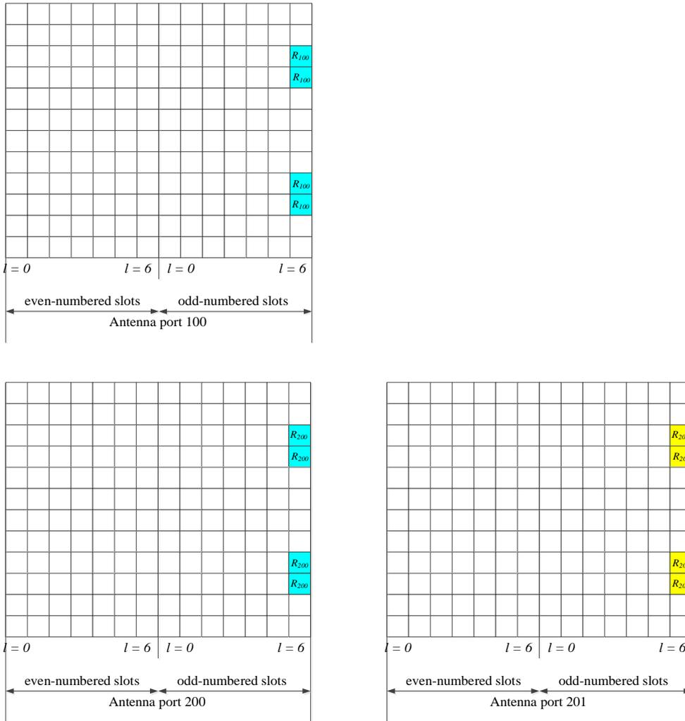
**Figure 5.5.2.2-1: Mapping of xPUCCH demodulation reference signals**
