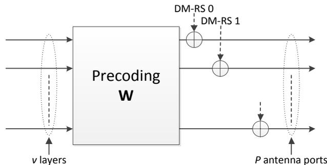
**Figure 5.3.3A.2-1: DM-RS location for transmit diversity**
