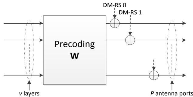
Figure 6.3.4.2-1: DM-RS location for transmit diversity
