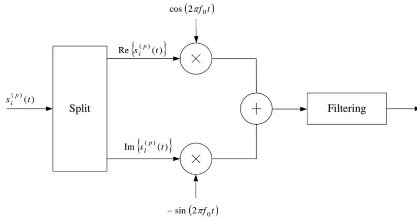
Figure 6.10-1: Downlink modulation
