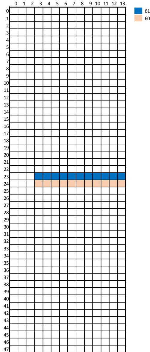
Figure 6.7.6.1-1: Mapping of phase noise compensation reference signals, antenna ports 60 and 61 in case of  $l_{first}^{xPDSCH} = 3$  and  $l_{last}^{xPDSCH} = 13$ .
