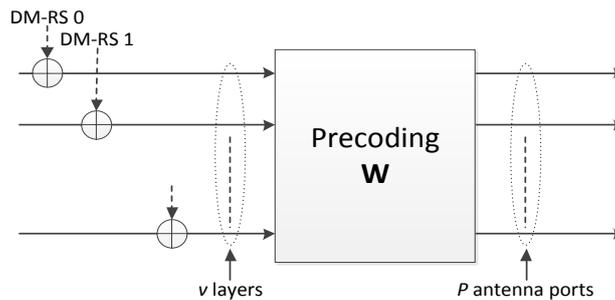
**Figure 5.3.3A.3-3: DM-RS location for spatial multiplexing using antenna ports with UE-specific reference signals**
