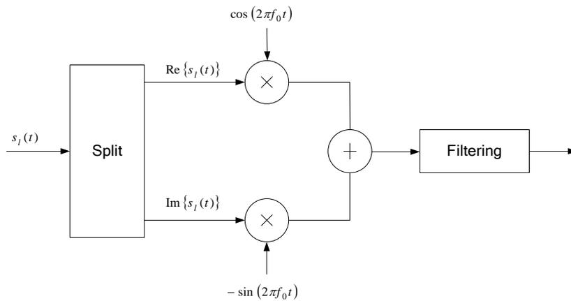
Figure 5.8-1: Uplink modulation
