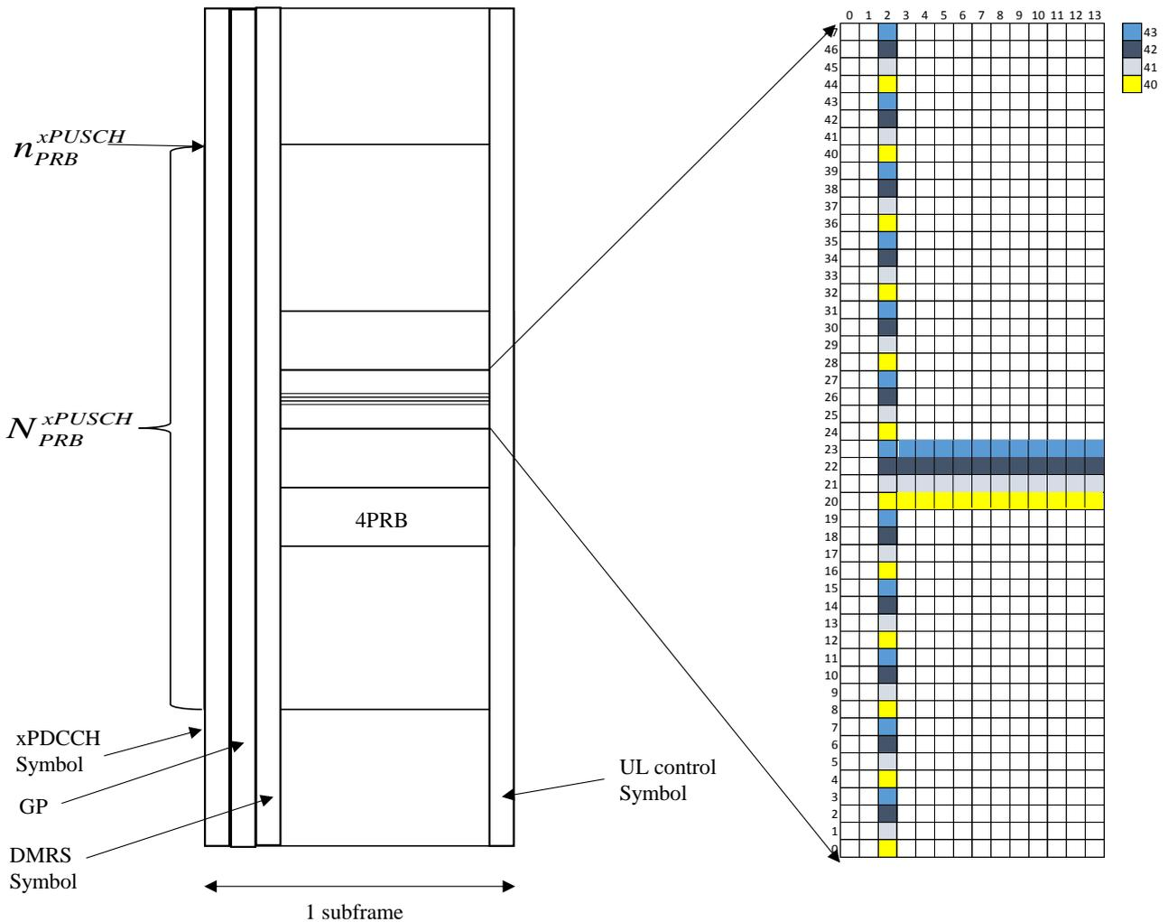
Figure 5.5.4.2-1: Mapping of phase noise compensation reference signals, antenna ports 50, 51, 52 and 53.
