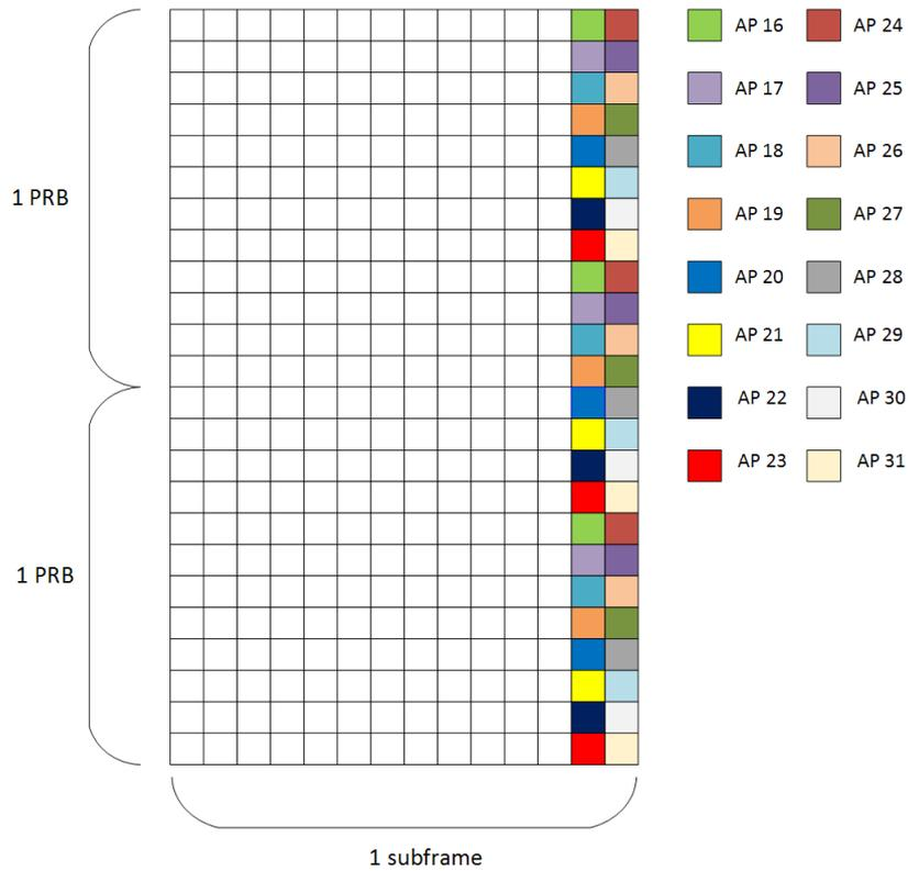
**Figure 6.7.3.2-1: Mapping of CSI-RS for 2 symbol allocation**
