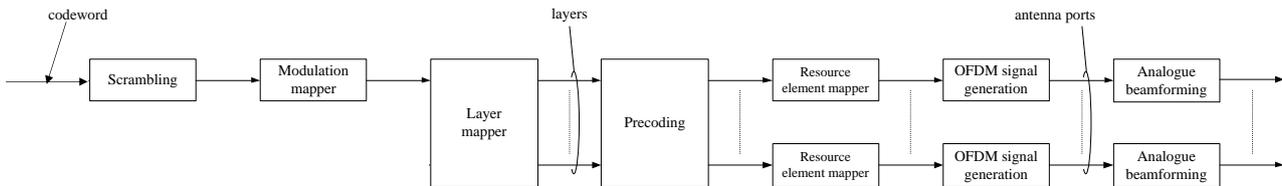
**Figure 5.3-1: Overview of uplink physical channel processing**
