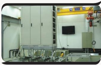
Picture of the Equipment Rack Base Isolation System Undergoing Earthquake Resistant Tests
